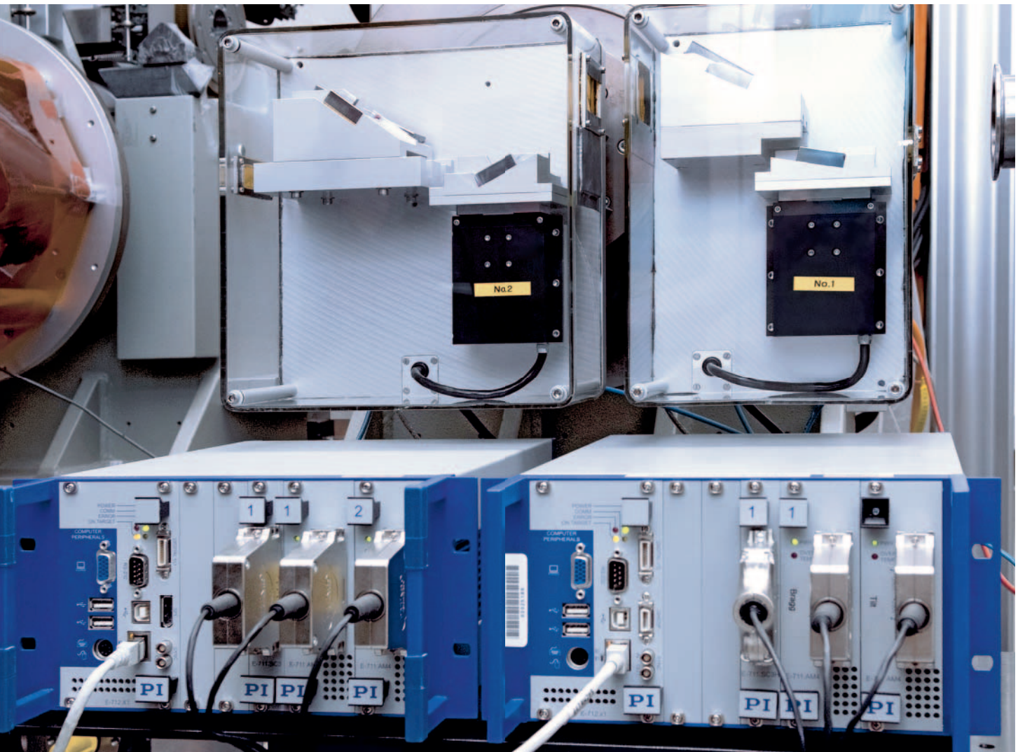
The two stages with PiezoWalk® drive and their controllers in the setup (Image: ESRF)
