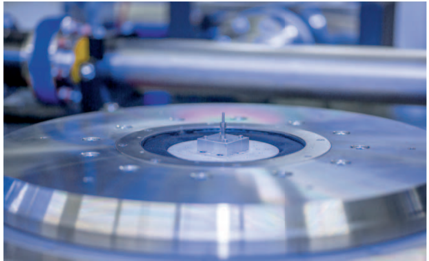
Ultra-precision sample positioning: Z stage, air-bearing rotation stage and a de-coupled 6-axis sample holder (left). The sample holder itself is located in the aperture of the rotation stage on the moving platform of a six-axis parallel kinematics (right) (Image: PI / HZG)
