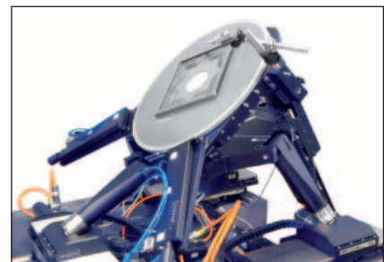
10-axis sample positioner, inclined 45° to the beam
