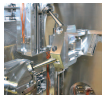
SpaceFAB advantage: A long stroke in X allows to place the platform with the lens outside of the beam
