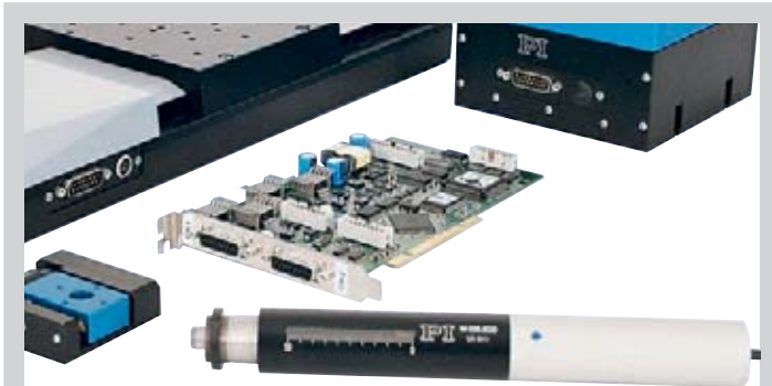
C-843.41 DC-motor controller board with M-110.DG linear stage, M-235.5DG heavy duty linear actuator, M-511.DD direct drive translation stage and M-501.1DG vertical stage. No external amplifier is required to drive any of these or other PI stages. Small motors are driven through the C-843's onboard linear amplifiers, direct-drive PI stages (e.g. M-511.DD) employ ActiveDrive™ controlled off the C-843's PWM outputs.
