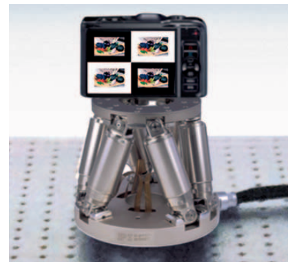
The H-811 Hexapod simulates camera shake for testing image stabilization systems according to the CIPA standard. Here in test equipment at Image Engineering. (Image: Image Engineering)
