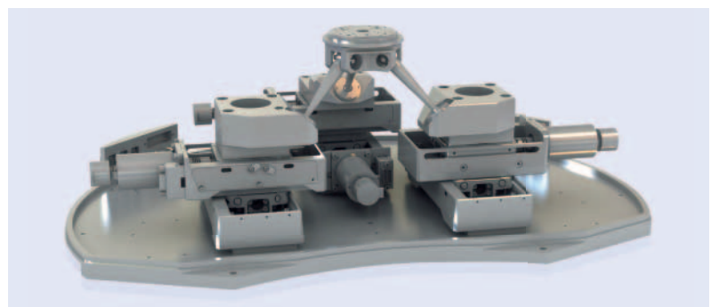
In this 3-strut design, additional degrees of freedom are produced because a passive strut can be moved in two or more axes. Example: In SpaceFAB, the individual struts are driven by one XY translation stage each
