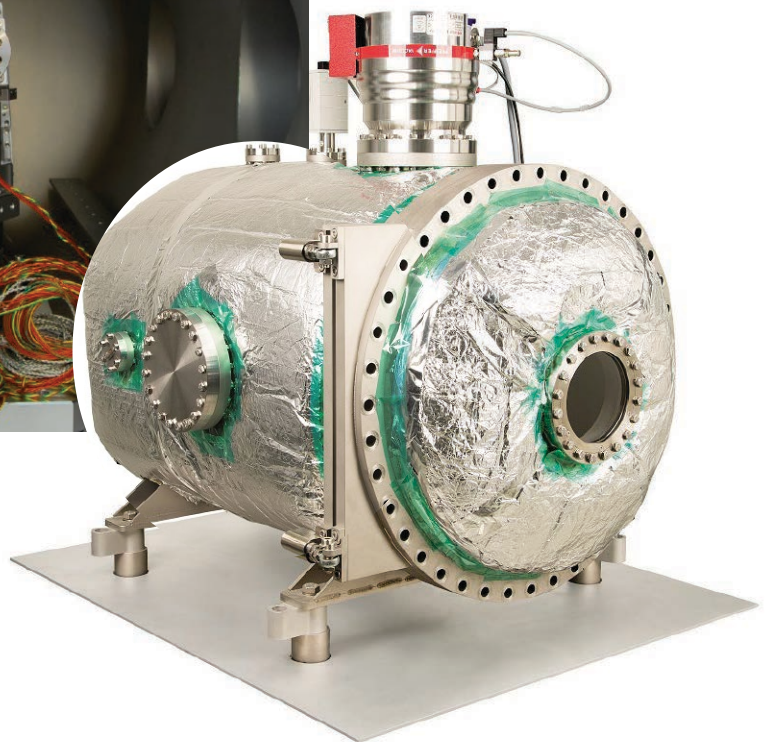
View in the vacuum chamber. Here, a multi-axis design awaits start-up and outgassing measurement
