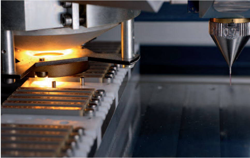
Automatic soldering machine with PICMA® actuators
