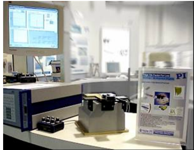
Figure 1. The OFC 2002 Collimator Alignment demonstration performed thousands of exacting collimator-collimator transverse/angular alignments right on the exhibition floor during the week of the conference.
