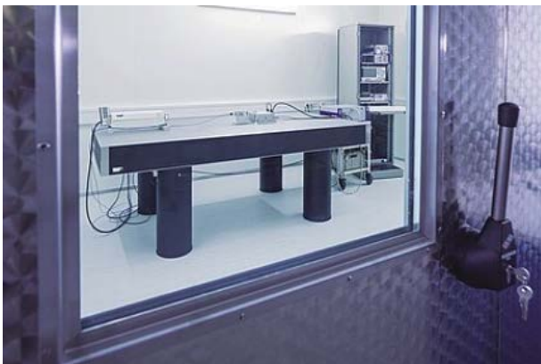
Fig. 1 View into a nanometrology laboratory with six-fold isolation. Measuring is done fully automatically under controlled ambient conditions.
