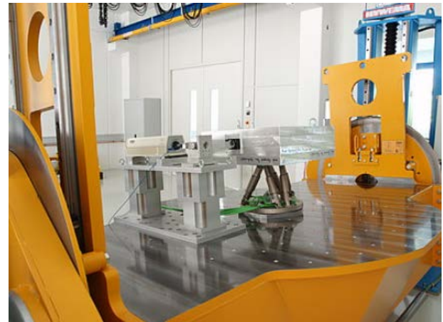
Fig. 5 At PI in Karlsruhe, lifting and tilting equipment specifically for measuring or qualifying products according to application is available. In this picture, a hexapod with load is measured interferometrically
