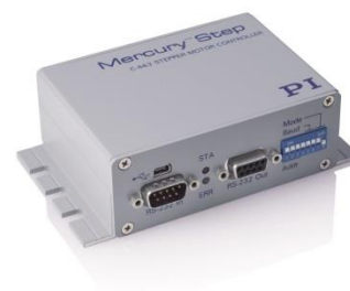
Fig. 34 C-663.11 Mercury Step; 16 microsteps per full step, without position control
