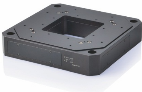
Fig. 5 The piezo-based scanning stage is essential for sample positioning. It is designed for working distances of 100 or 200 µm in the axes of the scanning plane and 30 µm in the Z axis. It allows a position resolution of better than 2 nm. Capacitive sensors and digital electronics provide maximum stability
