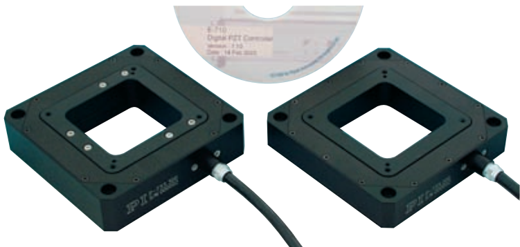
P-733.3 DD (left) and P-733.2 DD, high-speed, direct drive XY(Z) scanning stages are the fastest scanning stages with large aperture currently available (2.2 kHz resonant frequency!). Both units feature a footprint of only 100 x 100 mm. CD for size comparison.
