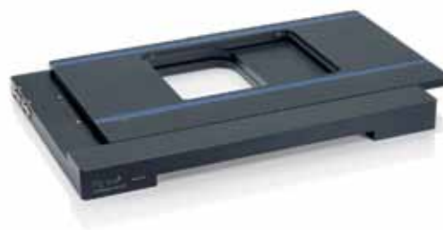
Customized M-686 stage with a bigger footprint makes it possible to sink the piezo Z scanner. The system height together with the P-541 piezo scanner is reduced to only 33 mm.
