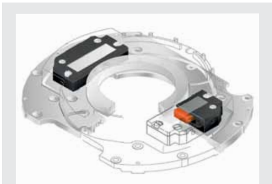
Implementation of rotary motion: PLine® motors act on a ring-shaped runner
