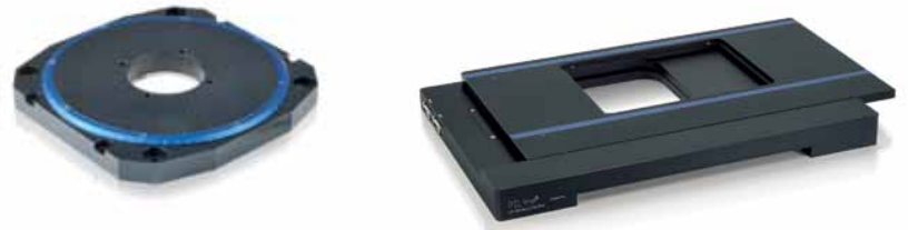
The benefit of the low profile PLine® drives becomes apparent with positioning systems such as the M-660 rotation stage (left, 14 mm high) or the M-687 microscopy XY stage (right, 25 mm high): a consistently flat design without lead screw ducts or flanged motors
