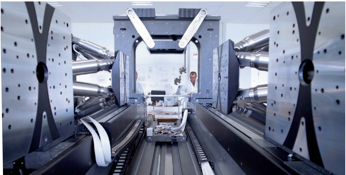
This 20-ton, 56-axis motion system is used for x-ray microscopy and quality assurance of x-ray optics. It is equipped with 56 motors, 16 controllers, 7 air bearing granite sliders and has an overall mass of more than 20,000 kilograms. An extraordinary precision of some hundreds of nanometers over the full range could be achieved.
