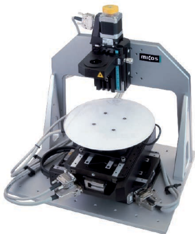
Wafer inspection system with integrated linear motor axes for fast precision XY scanning. Stepper motor axis for fine vertical position of the inspection equipment. Front page: Double-sided wafer inspection system in a flexible 15-axis configuration
