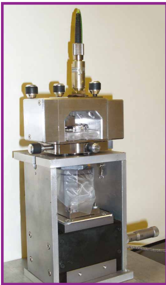
Figure 2. The apparatus stretches the molecule between a gold surface and the tip of a microscopic cantilever. Courtesy of Fernandez Lab.
