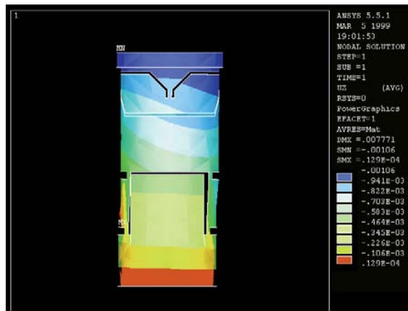
FEA stress simulation showing wire-EDM-cut flexure joint of a tip/tilt mirror system for astronomical telescopes
