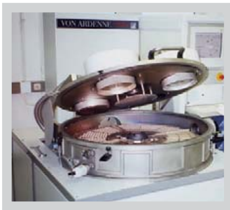
High-Tech manufacturing: Vacuum coating (sputtering) of piezo ceramics
