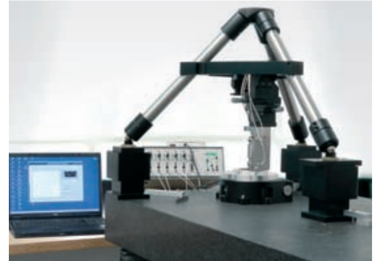
Angle measurement of evenness and eccentricity of rotation stages
