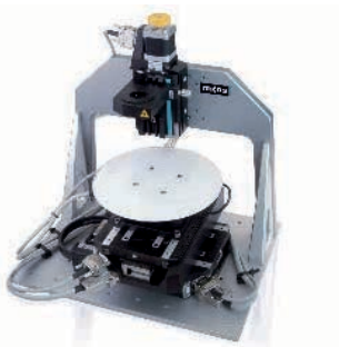
Wafer inspection system with integrated linear motor axes for fast precision XY scanning. Stepper motor axis for fine vertical position of the inspection equipment
