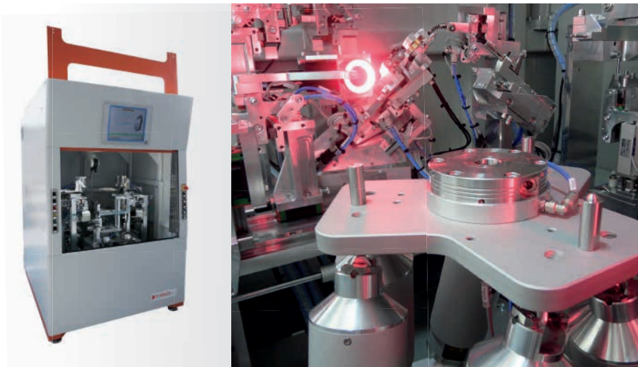
The hexapod systems make it possible to reduce the installation area for the robotics considerably (Image: DYMACO GROUP)
