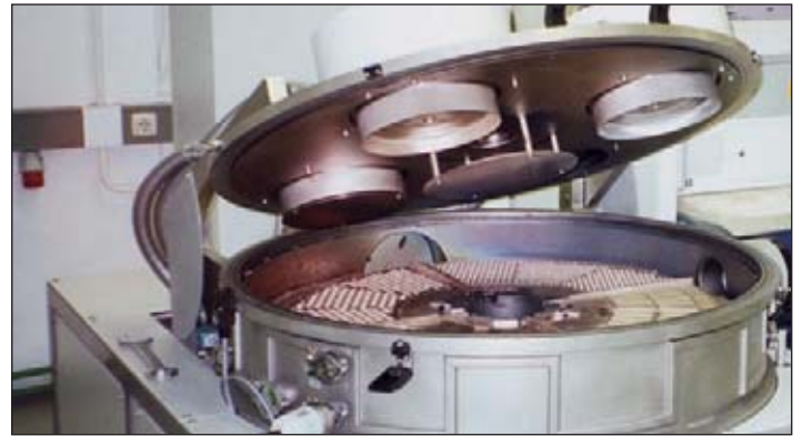
Sputtering facility at PI Ceramic
