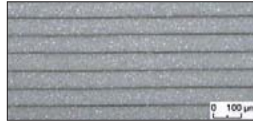
Piezoceramic layers in a monolithic actuator (LVPZT).
